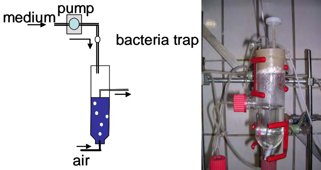
**Fig. 6: Chemostat system used for competition experiments and all other chemostat experiments described in chapter II - IV.** Left column show a simplified scheme of a one-stage-chemostat system. Right column shows a picture of an one-stage-chemostat reactor.
