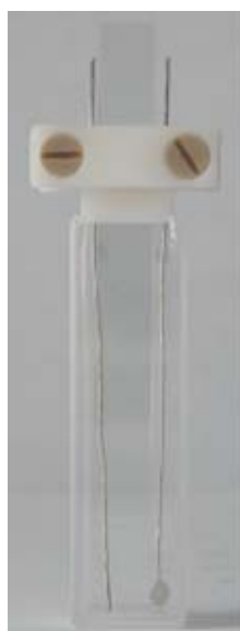
Figure 3.7 Three-electrode cell used for electropolymerization.
