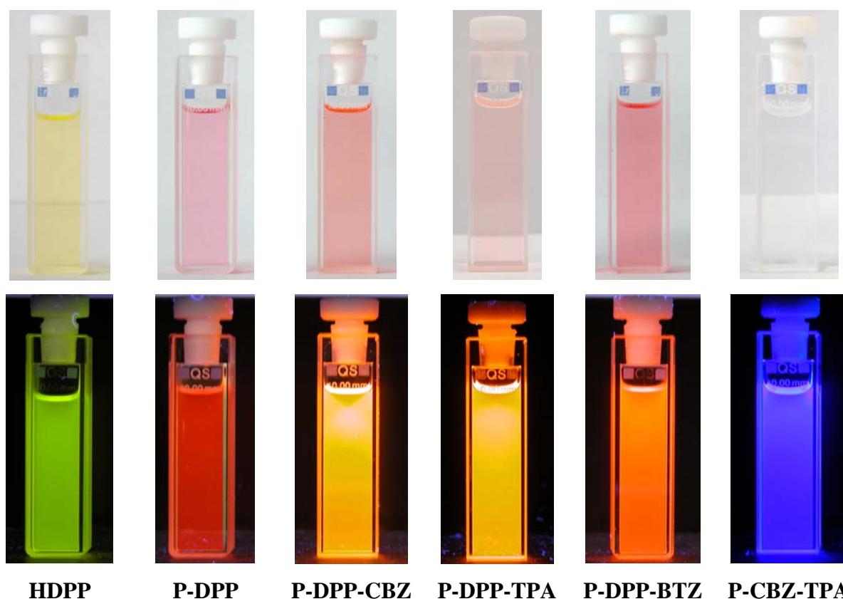
Figure 2.6 Photographs of HDPP and various polymers prepared via Suzuki polycondensation in normal (upper) and luminescent state (lower).
