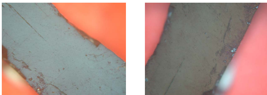
Figure 3.67: Polarization microscopy indicating single crystallinity for the \text{VO}_2 crystal HR151.
