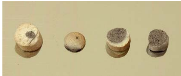
Figure 3.8: Parts of an inhomogeneously oxidized \text{YTiO}_3 bar due to sintering in a chamber furnace.
