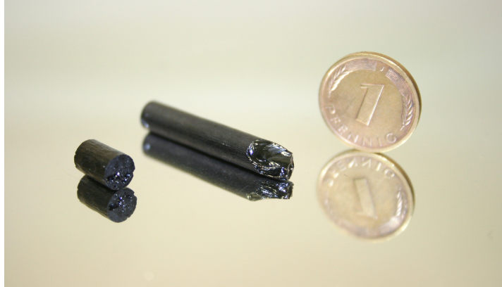
Figure 3.40: Parts of the crystals HR99 and HR141. The crystal HR99 exhibits a lot of cracks and splits very easily, while the crystal HR141 is a compact single crystal as an result of an optimized oxygen content.
