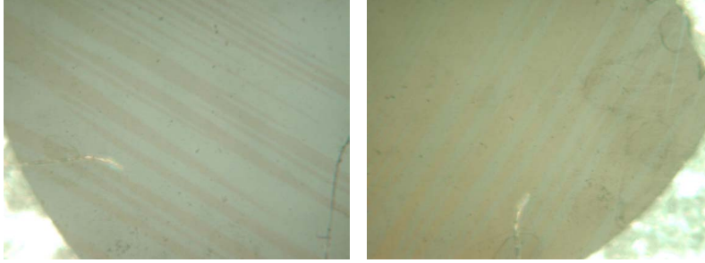
Figure 3.26: Strip-like domain pattern of the LaTiO 3 sample HR92-2 observed via polarization microscopy. In the right picture the sample was turned 90° hence the light stripes become dark, indicating different domain orientation.
