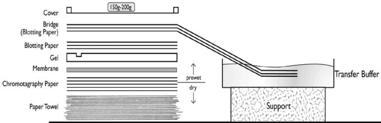
**Fig. 6: Setup of downward capillary transfer**
