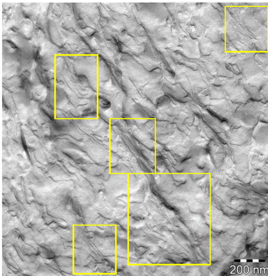
Figure 6.4: FFEM image of the system \text{H}_2\text{O}/(\text{sucrose}/\text{trehalose}) - \text{C}_6\text{MA} - \text{Agnique PG 264-G}/\text{Lutensol AO8} with \alpha = 0.4125 , \delta = 0.93 , \Psi = 0.75 , \zeta = 0.38 and \gamma = 0.12 . Not the expected bicontinuous structure but a lamellar phase is found.
