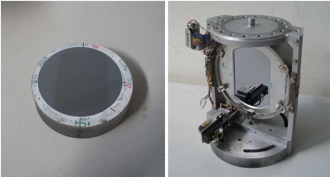
Figure 4.12: Left: Silicon Bragg crystal "Z13". Right: Crystal support and crystal with an aperture of 60mm width. On the bottom left a servo-motor with a linear potentiometer to adjust the crystal tilt.
