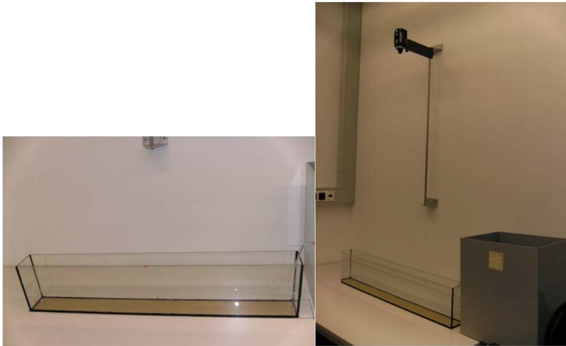
Fig. 23. Behavioral assay setup. (right picture): Complete behavioral assay with glass tank, stimulus application setup (gray box) and high definition video camera for recording zebrafish movement. (left picture): Fish tank ( 100 \times 10 \times 20 cm) with stimulus application tube on right side.
