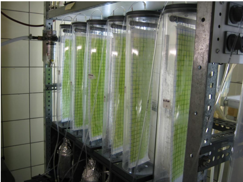
Figure 2-11. Bench-scale twin-layer system with 0.5 meter PMMA tube, from left to right Euglena gracilis (tube 1-3) and Chlorella protothecoides (tube 4-6)
