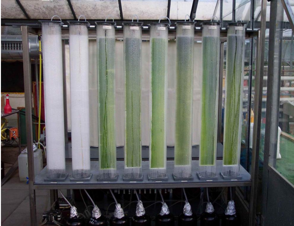
Figure 2-10. Bench-scale twin-layer system with 1 meter PMMA tube, from left to right, control (tube 1, 2), Chlorella vulgaris (tube 3-5) and Scenedesmus rubescens (tube 6-8)
