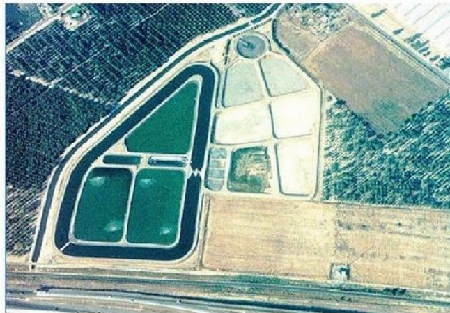
Figure 1-2. An Advanced Integrated Wastewater Pond Facility at Delhi, California, the USA ( http://ponce.sdsu.edu/aiwps.html )
