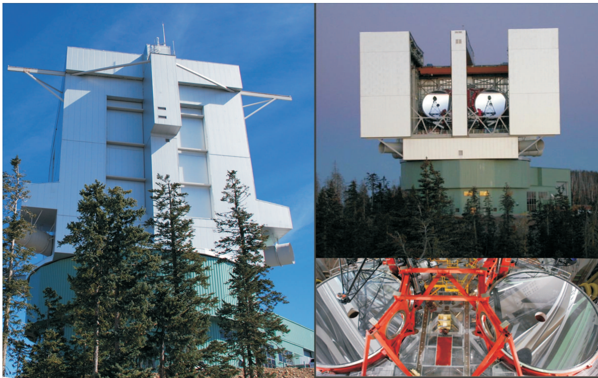
Figure 5.5: The Large Binocular Telescope uses an elevation over an azimuth mounting. The two 8.4 meter diameter primary mirrors are mounted with a 14.4 m center-center separation. By using swing arms to rotate the secondary mirrors and their supports, it is possible to switch the telescope from one mode of observation to another very quickly. The short focal length of the primary mirrors ( F/1.142 ) permits a compact, and therefore quite stiff telescope structure. Its construction began at July 1996 and the first light was on October 2005. Updates about the telescope and its instruments can be found in the official webpage: http://lbtwww.arcetri.astro.it/observatory_status.htm
