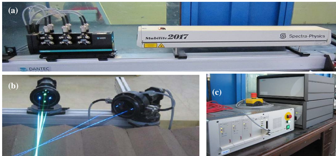
Figure 3-5: Appearance of the PDPA (by Dantec). (a) Laser generator; (b) Probes (laser transmitter and receiver); (c) Signal processor.
