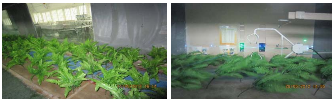
Figure 4-16: Surface with artificial trees tested in the wind-tunnel experiments.
