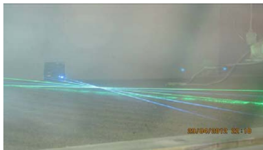
Figure 4-11: Deposition measurement over the sand surface.
