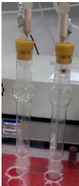
Figure 2.1: Glass vessels for CO 2 supplementation. The sterile filtered air/CO 2 -mixture was lead into the culture via thin glass tubes. The culture volume for optimal mixing was 25 ml.
