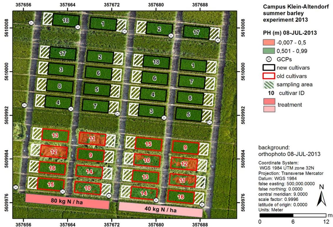
**Figure 8-6: Lodging detection based on PH at the summer barley study site Campus Klein-Altendorf, Rheinbach, 08 July 2013, GCPs = ground control points used for CSM generation.**
