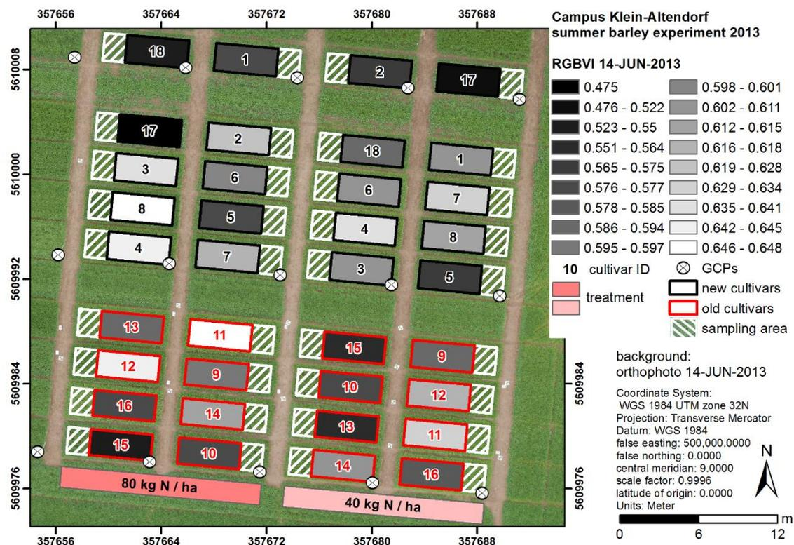
**Figure 8-5: Cultivar discrimination based on RGBVI at the summer barley study site Campus Klein-Altendorf, Rheinbach, 14 June 2013, GCPs = ground control points used for CSM generation.**
