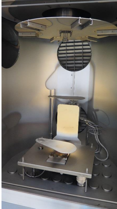
Fig. 3.3: Picture of the evaporation setup of the Helmholtz Nanoelectronic Facility (HNF) of Jülich Research Center.
