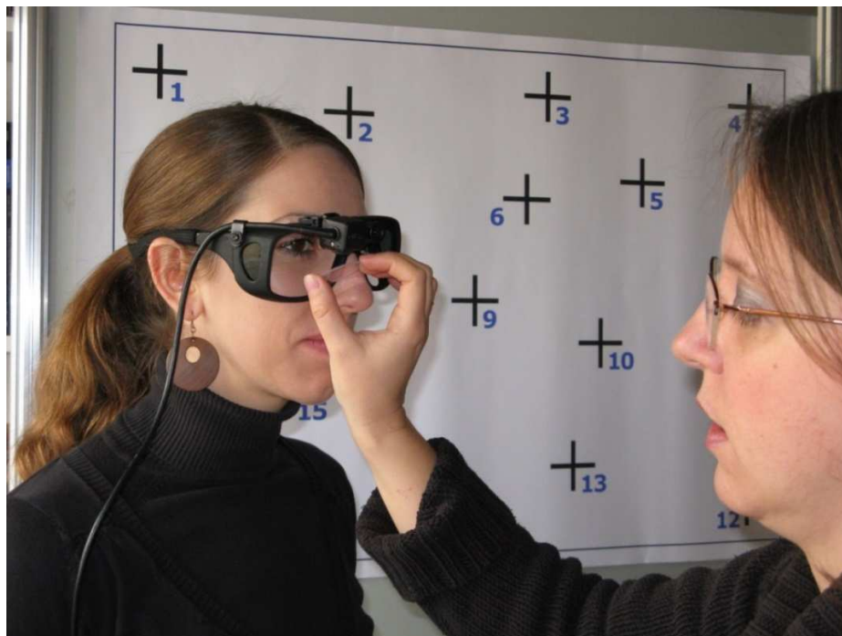
Figure 1: Calibration of the ASL MobileEye (copyright by Kira Eghbal-Azar)
