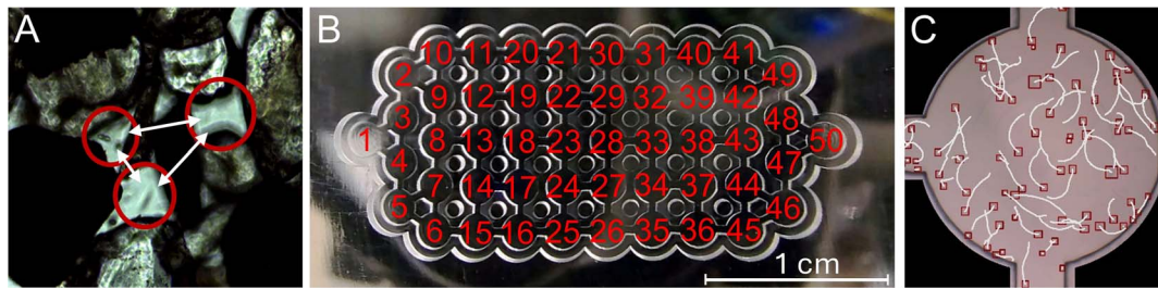
Figure 2. Experimental design of the microfluidic chip. (A) Microscopic image of ciliates from the interstitial region of a sandy beach (Helgoland Island, North Sea, Germany), serving as an ecological reference for distinct environmental patches, analogous to those in our microfluidic chip. (B) The microfluidic chip with all chambers numbered as used later in the presentation of results. (C) Video-view of a microfluidic chip habitat patch, highlighting ciliate cells with squares and their movement trajectories. For further details, see Methods section.
