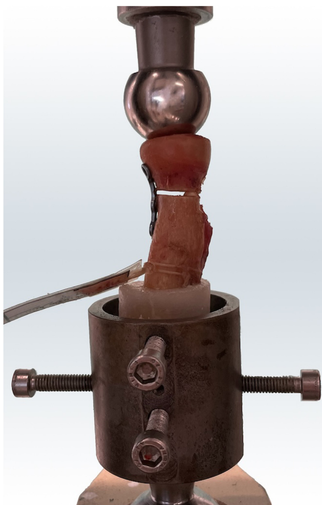
Figure 4 Proximal radius with plate fixation and bone graft placed in the test machine for testing.
