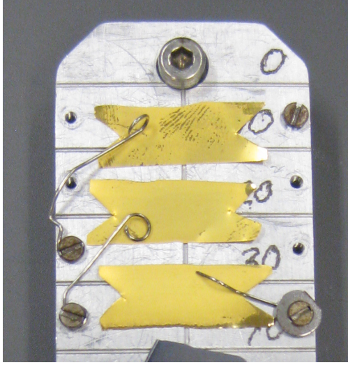
Figure 4.1: Three RbCl targets on the target ladder for RBS measurements at the RUBION facility in Bochum [222], in October 2013. The targets are consecutively numbered from one to three. There is a fingerprint clearly visible on target 1, wherefore targets 2 and 3 were used in experimental campaigns.
