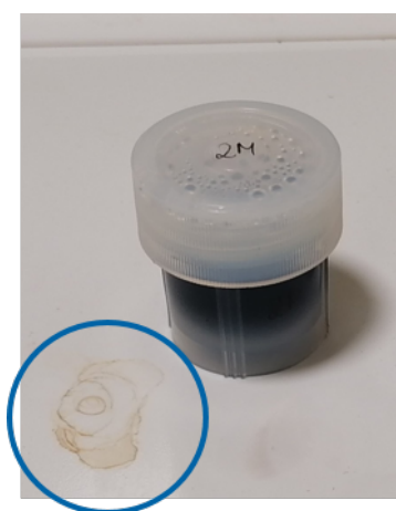
Figure 3.3.: Picture showing the PFA vessel of sample “15 M_ash” shortly after the partial spillage of sample solution from the “closed” PFA vessel onto the hot plate. The blue circle highlights the dried residue of the spilled sample solution on the hot plate. This resulted in a measured ^{90}\text{Sr}/\text{Sr} ratio that was significantly higher than the information value of the IAEA-447 sample material [100].
