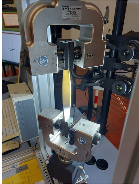
Figure 6.11: Setup of the torsion experiment. The photograph is provided courtesy of the Institute for Frontier Materials on Earth and in Space at German Aerospace Center (DLR). The photograph has been taken by Max Zinke.
