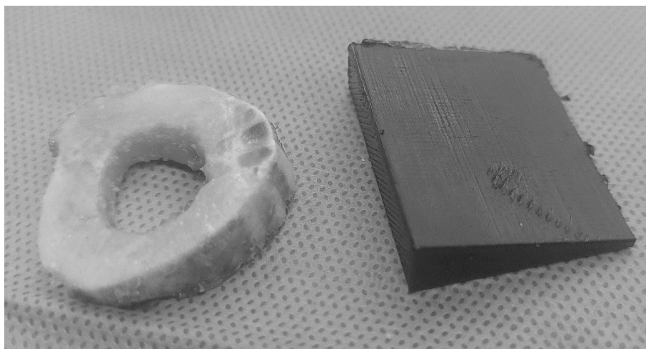
Fig. 2. Customized crafted bone wedge (left) and 3D-printed PLA wedge (right).
