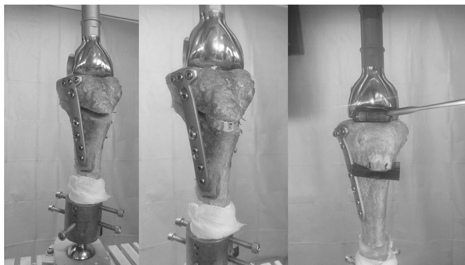
Fig. 1. Biomechanical testing setup; locking plate alone (left); locking plate with additive bony wedge (middle); locking plate with additive 3D-printed PLA wedge, adjusted with a spirit level (right).
