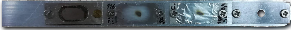
Figure 3.3: Occupancy of the target ladder of SONIC during the experiments. From left to right: ^{56}\text{Co} source, ^{116}\text{Sn} target, ^{118}\text{Sn} target and 3 mm aperture for beam focusing. The dimension of one of the target frames is 2.5 \times 0.9 \text{ cm}^2 . The beam spots in the center of the targets are clearly visible. The target ladder is inserted vertically into the target chamber, with the aperture in the lowest position.
