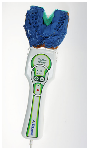
Fig. 1 Adapted piezoelectric T-scan sensor foil with individualised surface for measuring maximum bite force and bite force endurance over the entire dental arch
