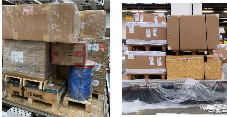
Fig. 2. Air cargo PLP: Strong heterogeneity of items during buildup in an air cargo hub. Most items are boxes or box-shaped, and some are attached to a wooden subpallet. The layout contour can take various forms, for example, cuboidal when placed in the middle of the aircraft main deck or with cutouts when placed next to the rounded aircraft sides.
