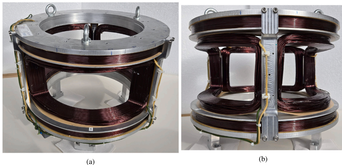
Fig. 10. Set of Helmholtz coils allowing one to apply a magnetic guide field of 2 mT in any direction for longitudinal polarization analysis.
