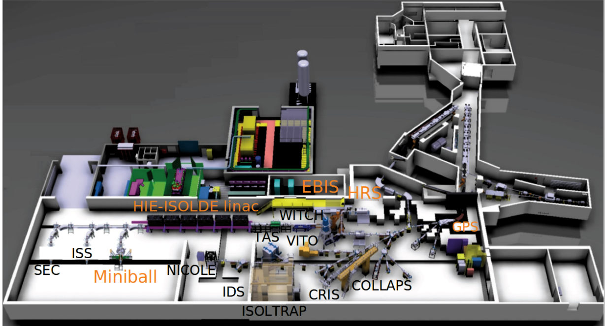
Figure 3.1. Schematic layout of the ISOLDE hall, highlighting the GPS and HRS mass separators connected to two separate target stations. Components discussed in this thesis are marked in orange-red. Adapted and modified from Ref. [118] with kind permission of CERN.
