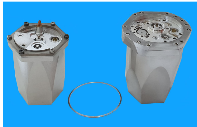
Fig. 6 The new encapsulation of the Miniball and AGATA HPGe detector is based on a metal-elastic seal between the capsule lid and the crystal container. A seal of the AGATA detector is shown between the two detectors. The delicate crystals can now be accessed in a replicable way by opening and closing the capsule in a controlled way
