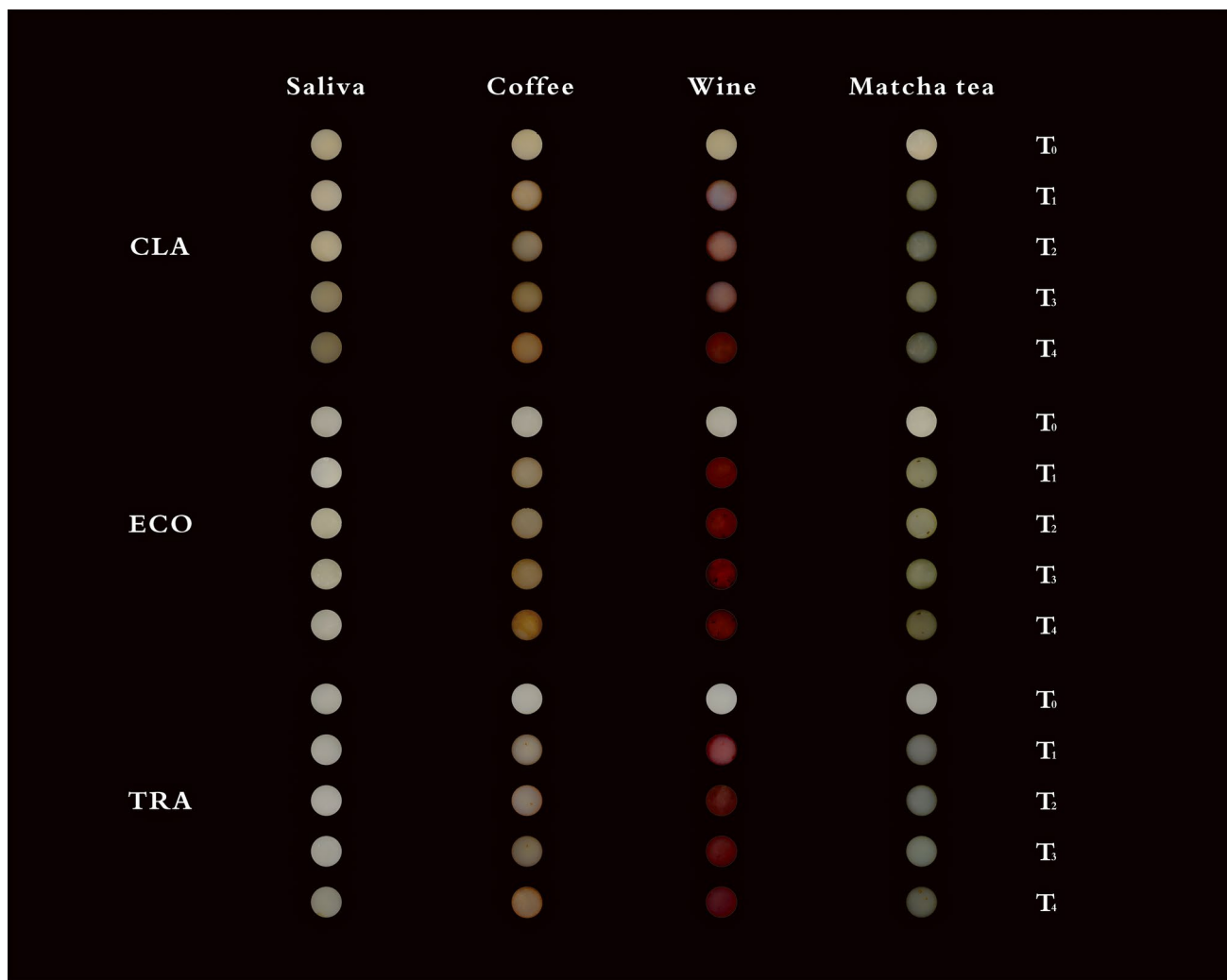
Fig. 2 Representative photographs of test specimens from each group after immersion in staining solutions, illustrating visual differences in discoloration. Abbreviations: ECO, Ecosite One; TRA, Tran-
