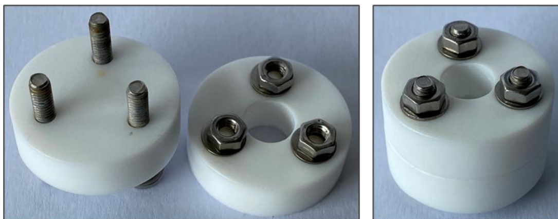
Figure 67: Photograph of the sedimentation cell used for thin-target preparation, shown disassembled (left) and assembled (right).
