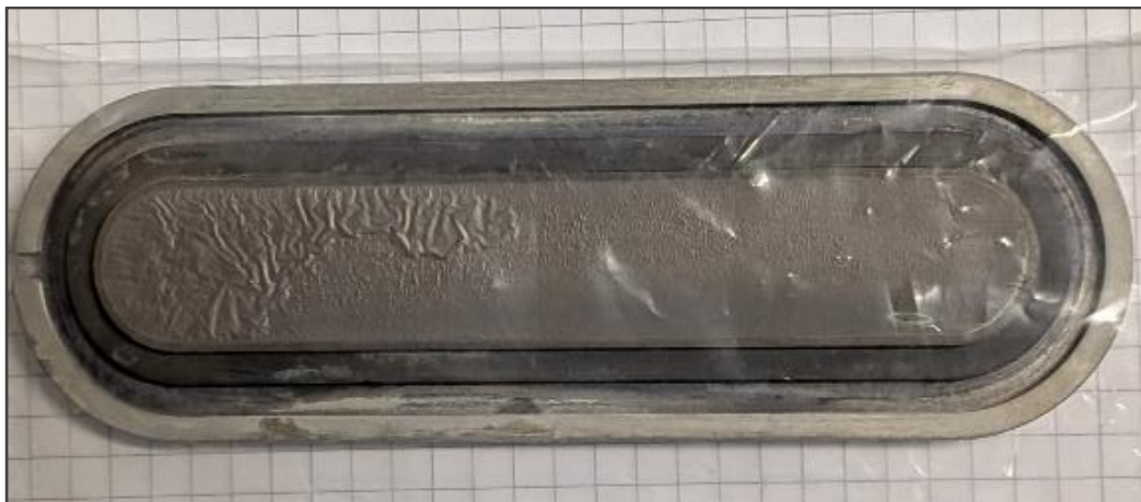
Figure B-3: Original photograph of a bismuth target processed in a vertical oven DD assembly as presented in Section 3.2.2
