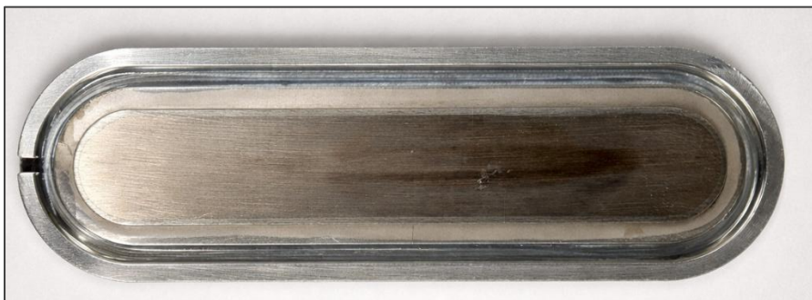
Figure 31: Photograph of a target prepared by melting technique after a 4 h irradiation showing slight abbreviation on the target surface roughly resembling the beam shape footprint. The photograph is edited to increase visually while maintaining radiation protection. The original photograph is shown in the appendix in Figure B-1.
