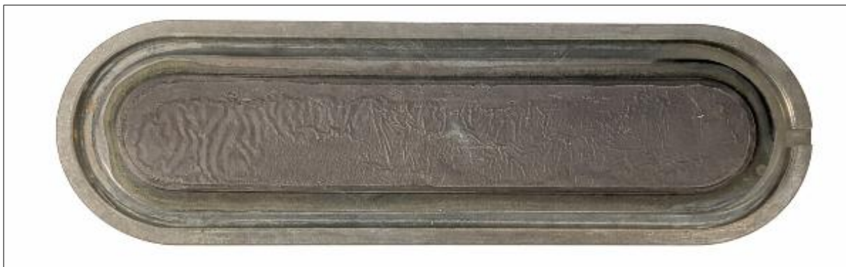
Figure 47: Showing a bismuth target after irradiation and after dry distillation processing using a vertical oven setup at 570 °C. Photographs is visually cleaned. The original photograph is shown in the Appendix in Figure B-3.
