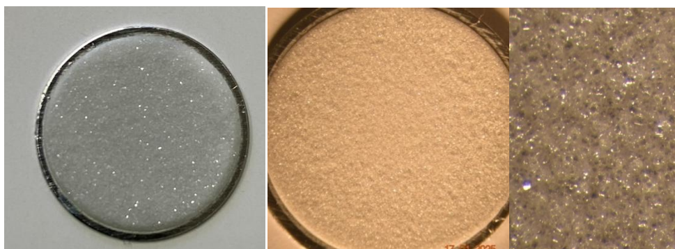
Figure 70: Photograph of a representative As 2 O 3 target prepared by manual vapor deposition on an aluminum backing (magnified by ~1.5 x (A), ~2 x (B) and ~10 x (C))
