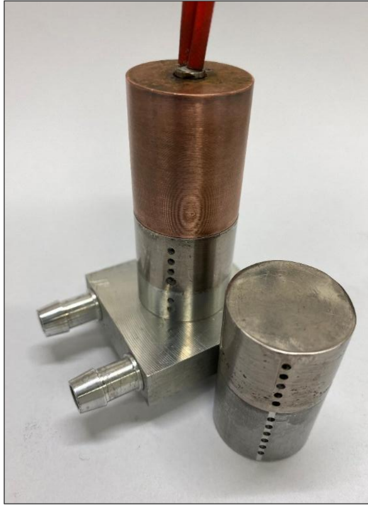
Figure 73: Photograph of the two Bi/Al test rods used for the experimental determination of the effective thermal contact resistance between bismuth and aluminum for target preparation routes.
