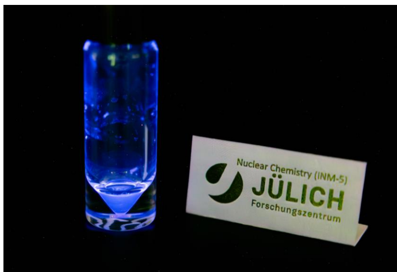
Figure 54: Long-exposure photograph of a ^{211}\text{At} -containing vial showing localized blue emission along the vial wall and near residual activity deposits. The spatially localized pattern supports a surface-related radioluminescence contribution rather than a purely homogeneous gas-phase emission. (photograph by Dr. Alexander Haseloer)
