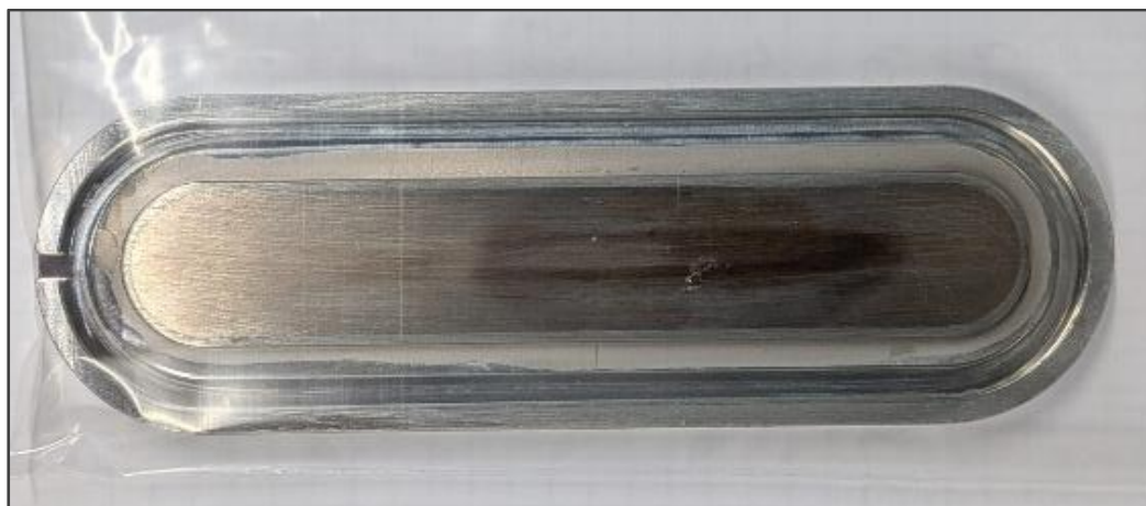
Figure B-2: Unedited photograph of the target presented in Section 3.2.1, showing a bismuth target prepared by melting technique, irradiated for \sim 4 h with \sim 50 \mu\text{A}_e .
