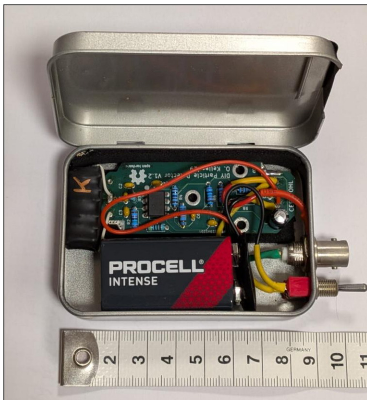
Figure B-7: Auxiliary low-cost PIN-diode detector setup used for supplementary qualitative count-rate observations. The detector concept was based on Keller et al. [123], while the Python-based data-acquisition script was provided by a colleague. The setup was not used for traceable absolute activity quantification in this thesis.
