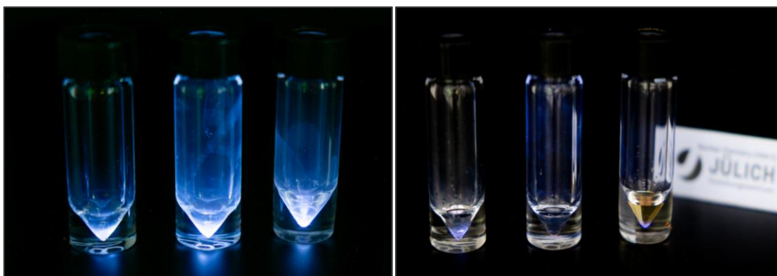
Figure 53: Long-exposure photographs of ^{211}\text{At} -containing V-vials under different gas and solvent conditions. (A) Dried ^{211}\text{At} samples under argon, helium, and krypton atmospheres. (B) Corresponding samples after addition of water, chloroform, or diiodomethane. The images show that the visible emission persisted under different atmospheres but decreased markedly after addition of liquid, with the spatial emission pattern depending strongly on the apparent activity distribution (photograph by Dr. Alexander Haseloer).
