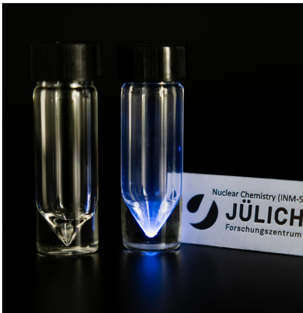
Figure 52: Showing a long-time exposure photograph (2 min) of radioluminescence of ^{211}\text{At} (~3 GBq) in a V-shaped borosilicate glass vial (right). As comparison, a similar vial without activity is shown right beside (left). The radiation dose measured of this assembly was \sim 57 \text{ mSv h}^{-1} contact dose and \sim 600 \mu\text{Sv h}^{-1} at 30 cm distance (Camera distance). The radiochemical preparation was performed by Lucas Mues (Author) whereas the photograph was taken by Dr. Alexander Haseloer.
