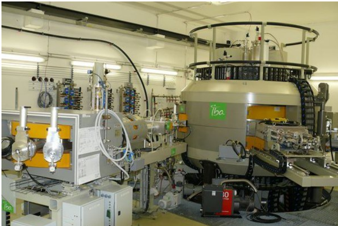
Figure 5.11: The Cyclone 30XP cyclotron facility at the INM-5, used for radionuclide production and target irradiation [74].
