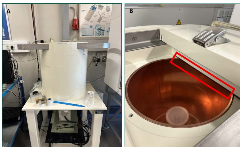
Figure 3.3: BEGe detector system used for gamma-ray spectrometry measurements. The detector was housed in a lead shield (A), and the principal counting geometry was defined by a source-to-endcap distance of 19 cm (B).
