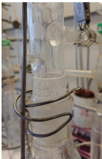
Figure 4.21. Sublimate obtained from a reaction between one equivalent of [\text{Zr}(\text{NEt}_2)_4] and two equivalents of H -TFB-TFEA in n -heptane.
