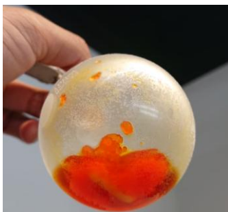
Figure 4.10. As-obtained [\text{Zr}(\text{TFB-}t\text{BuA})_2(\text{NEt}_2)_2] upon recrystallization in a mixture of toluene and n -heptane stored at -20\text{ }^\circ\text{C} .
