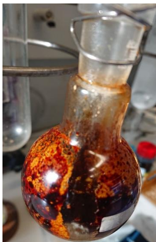
Figure 4.14. [Zr(TFB- t BuA) 2 (NEt 2 ) 2 ] after sublimation attempt approximately 100 °C ( p \approx 1 mbar).
