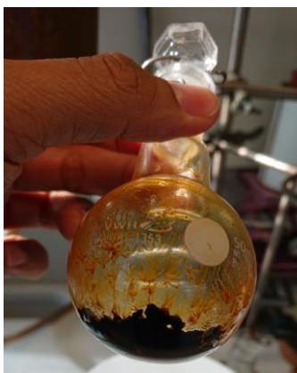
Figure 4.8. [\text{Zr}(\text{TFB-MEA})_2(\text{NEt}_2)_2] after sublimation experiment at approximately 100 °C ( p \approx 1 mbar).
