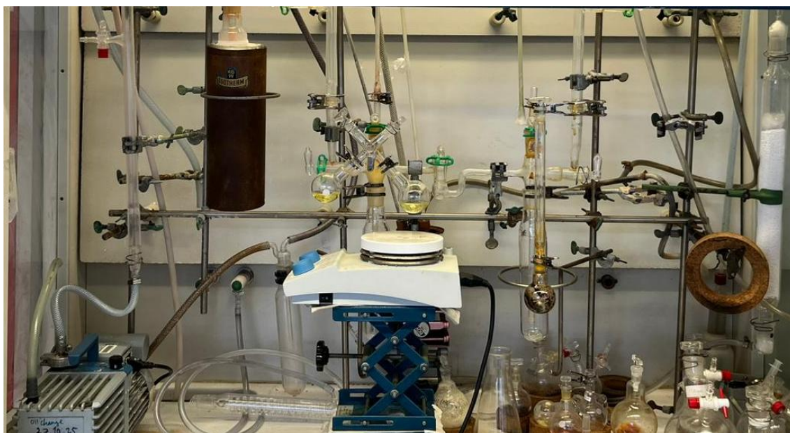
Figure 7.1. Stock line setup for inert condition reaction.
