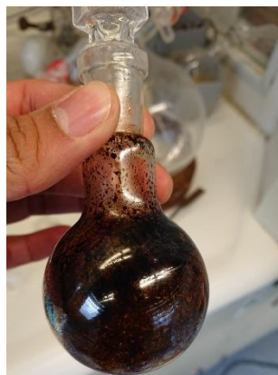
Figure 4.19. [\text{Zr}(\text{TFB-}t\text{BuA})_2\{\eta^2\text{-(}i\text{PrN)}_2\text{CNEt}_2\}_2] after sublimation attempt at approximately 100 °C ( p \approx 1 mbar).
