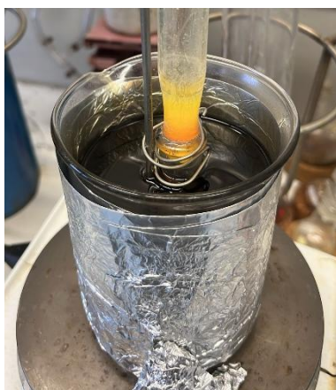
Figure 4.29. Sublimate obtained from a reaction between one equivalent of [\text{Zr}(\text{NEt}_2)_4] , one equivalent of \text{HO}^t\text{Bu} , and two equivalents of H -TFB- t BuA.
