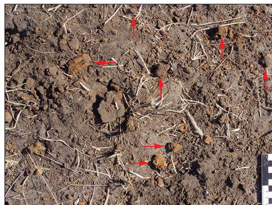
Figure 15: Plinthic iron oxide segregations (marked with red arrows) used in traditional smelting.
