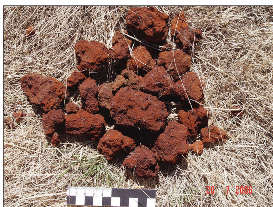
Figure 13: Plinthic iron ore concretions from the upper, red soil horizon of Figure 12. These nodules were used in historical smelting operations.
