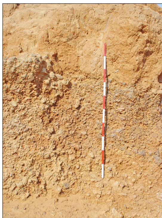
Figure 161: SC 48 Popa, area N07/04: soil section showing pisolitic ferricrete of the Omatako Formation.
