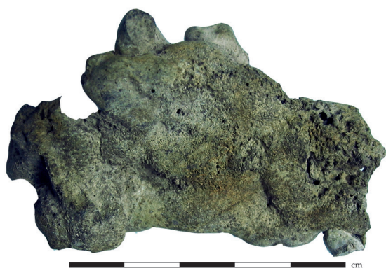
Figure 208: Ruuga (SC 3), area N98/39-1: sample 4388/06, flow slag that solidified along a furnace wall with some attached sediment.
