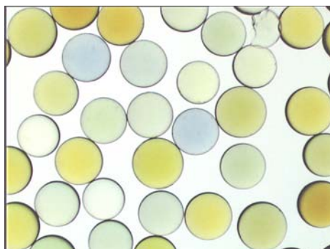
Figure 1-2: Microscope view of the solid-supported peptide–copper complexes.
