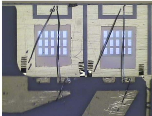
Figure 7-31 Matching network of the bond-wires [47]. The IF signal is fed into the acousto-optical crystal by means of a transducer array, which provides a couple of bonding possibilities. In the picture, the micro-strip boards correspond to channel 1 and 2 of the deflector. With the length of the parallel bond-wire the inductance can be matched to become low SWR.
