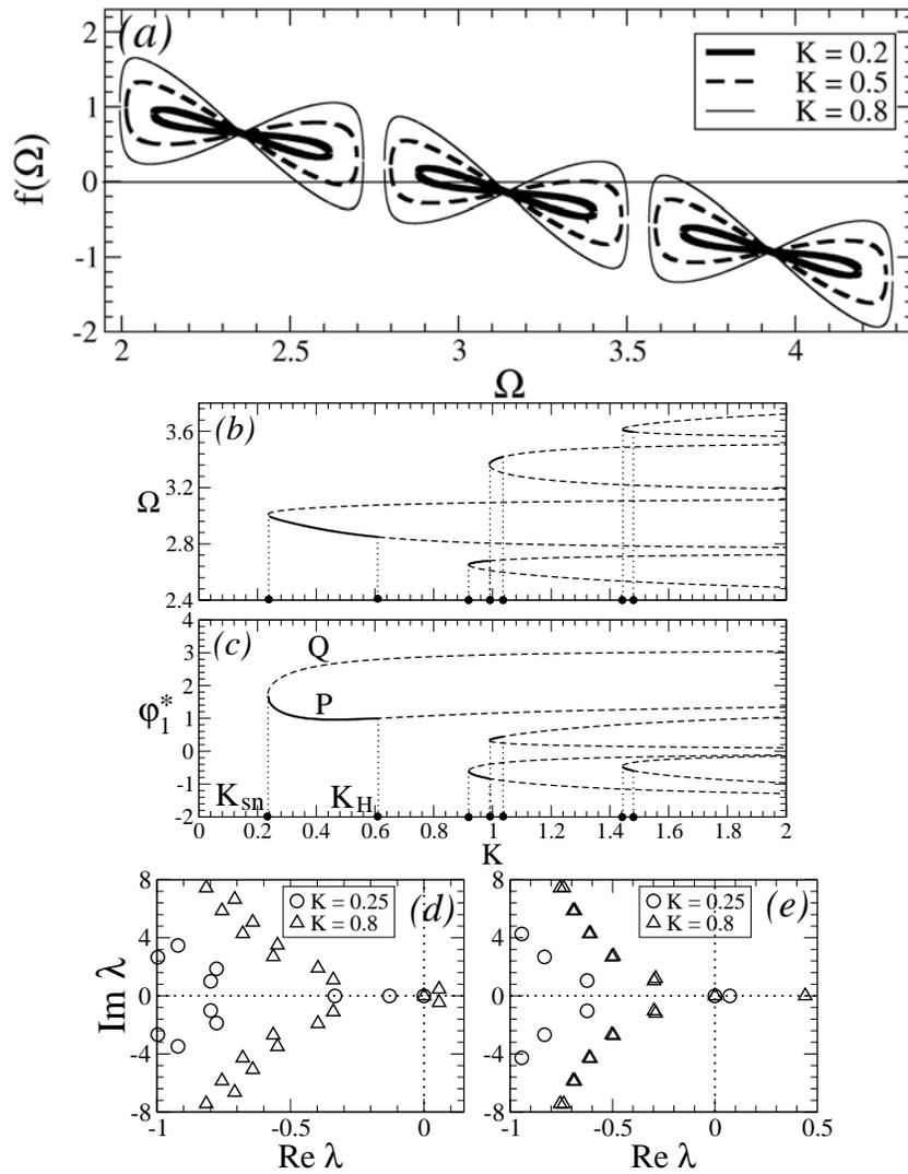
Figure 2.6: Phase-locked states of system (2.1). (a) Graphs of the function  $f(\Omega)$  (2.7) for three values of  $K$ . (b),(c) Phase-locked states  $(\Omega, \varphi_1^*)$  of system 2.1 appears in pairs. Stable ones are depicted by bold lines, unstable- by dashed lines. (d),(e) Eigenvalues for the fixed point  $P$ ,  $Q$ , respectively. Eigenvalues are shown for two coupling strength  $K = 0.25$  and  $K = 0.8$ . Parameters  $\Delta_1 = 0.2$ ,  $\Delta_2 = 3$ , and  $\tau = 4$ .
