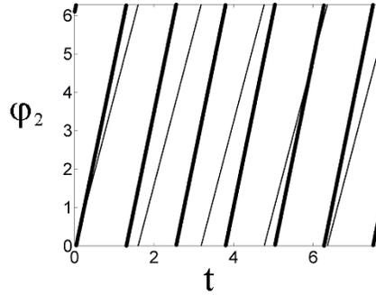
Figure 2.4: Coexistence of two stable in-phase-locked states  $P$  and  $P'$  with the same phase difference  $\varphi_1^* \equiv 0$ , but with the different frequencies  $\Omega_P = 5.12$  and  $\Omega_{P'} = 3.96$ , respectively. Time courses of the mean phase  $\varphi_2$  are shown for stable states  $P$  (bold line) and  $P'$  (thin line). Parameters  $\Delta_1 = 0.0$ ,  $\Delta_2 = 4.5$ ,  $\tau = 1.4$ , and  $K = 1.6$ .
