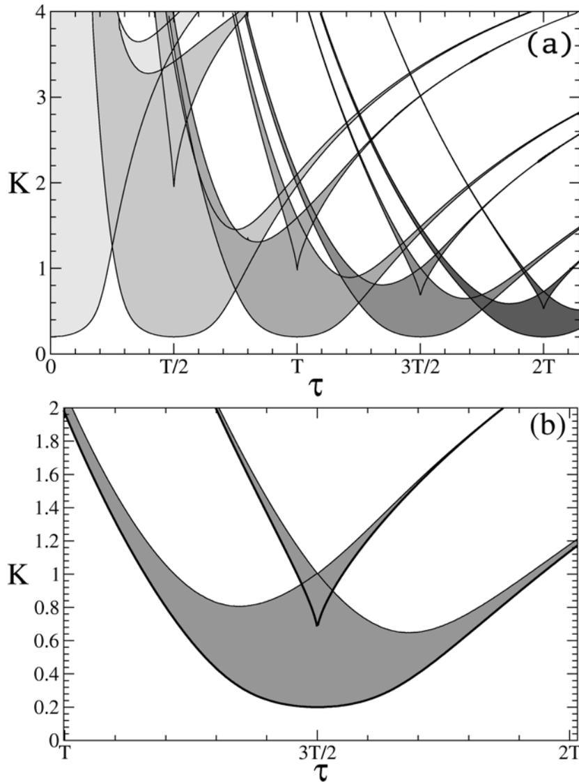
Figure 2.7: (a) The first five "swallows" of stability regions' family are shown. Each region of the same color starts from below with a curve of a birth of a stable phase-locked state and is bounded from above with a curve, when stable fixed point loses its stability. (b) One exemplary "swallow" is shown in details. Parameters  $\Delta_1 = 0.2$ ,  $\Delta_2 = 3.0$ .
