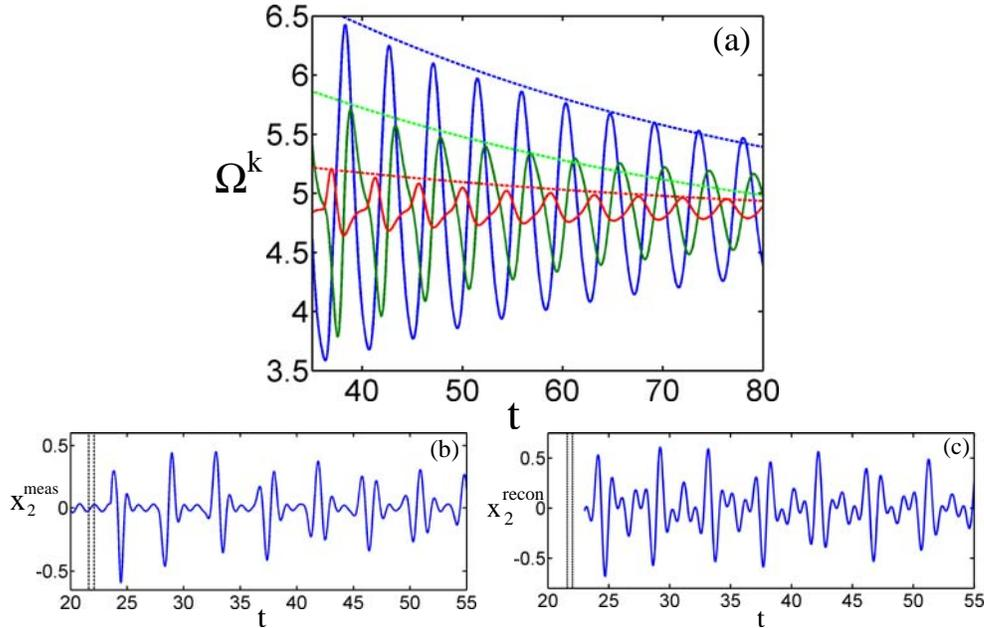
Figure 4.5: (a) Oscillations in frequencies of three exemplary trials in  $(\Omega_2, \alpha_2)$  phase-locked state after stimulus. Dashed curves provide envelope for amplitude decay. (b)  $x_2^2$  averaged signal as it results from the stimulation ("meas" stands for "measured"). (c)  $x_2^2$  averaged signal reconstructed using suggestions about frequencies of every trial. Parameters:  $\tau = 2$ ,  $\Delta_1 = 0.4$ ,  $\Delta_1 = 2\pi$ ,  $K = 9.7$ ,  $I = 100$  and  $\theta = 4.78$ .
