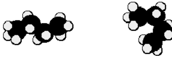
Figure 3.1. Trans (left) and cis (right) configurations in a segment of a polyethylene molecule. C atoms in the skeleton of the chain are shown in black, H atoms in grey.
