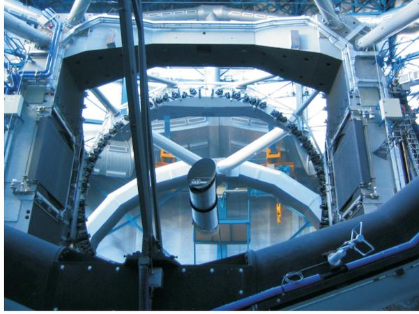
*Figure 2.4:* The main mirror on one of the four telescopes. It has a diameter of 8.2 meter. Also the Nasmyth mirror that directs the light to one of the foci can be seen.
