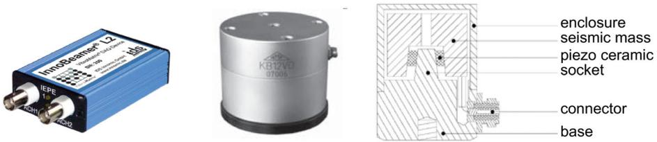
**Figure 2.7:** For the vibration measurement accelerometers based on the piezo-effect are used. A shear-force is applied to the piezo-ceramic, if the seismic mass is accelerated vertically, resulting in a voltage signal.
