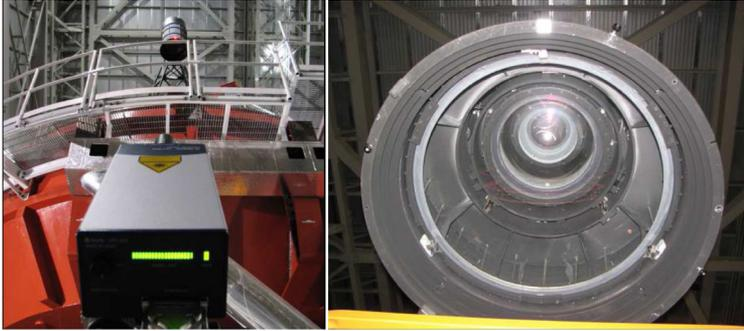
**Figure 2.8:** Vibration measurement of the LBT: A laser vibrometer is used in OPD direction to monitor intrinsic vibrations of the whole telescope structure relative to the dome building.
