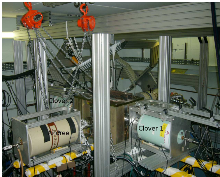
Figure 3.13: Experimental setup used for the g factor measurement at the Lohengrin mass separator in Grenoble.
