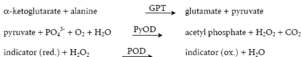
The change in indicator colour was detected by a photodiode element.
