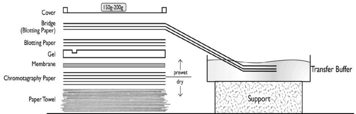
**Fig. 6: Setup of downward capillary transfer**
