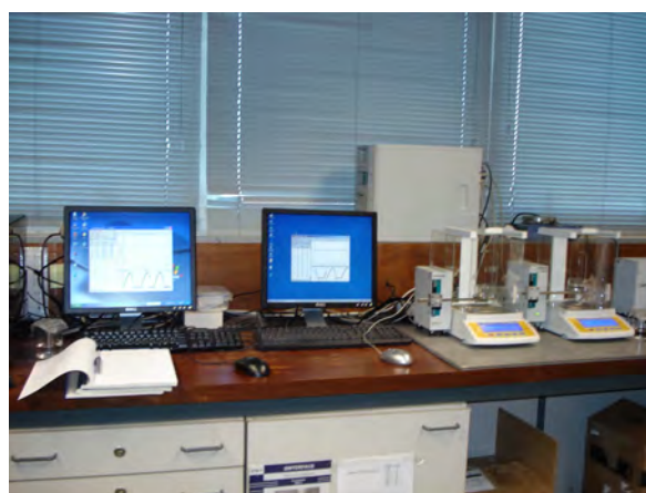
Fig. 2.11. The surface tension measurements equipment: the computer, the STA-1 tensiometer and the Sartorius balance.
