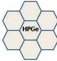
Figure 3.16: A schematic layout showing the arrangement of seven HPGe crystals in a common cryostat of a RISING cluster detector [47].
