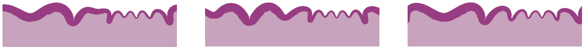
Figure 4.14: Snapshots of three different realizations of systems with the same parameters, T_0 = 0.278\text{cm} , A = 0.200\text{cm} , and \theta_g = 2.5 , and distinct random number generator seeds.
