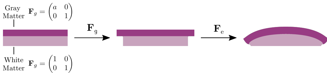
Figure 2.3: Effects of application of the growth tensors shown inside the figure. From left to right, the original, grown, and final configurations are shown. On the grown configuration \mathcal{B}_g the top layer grows tangentially by a factor a .
