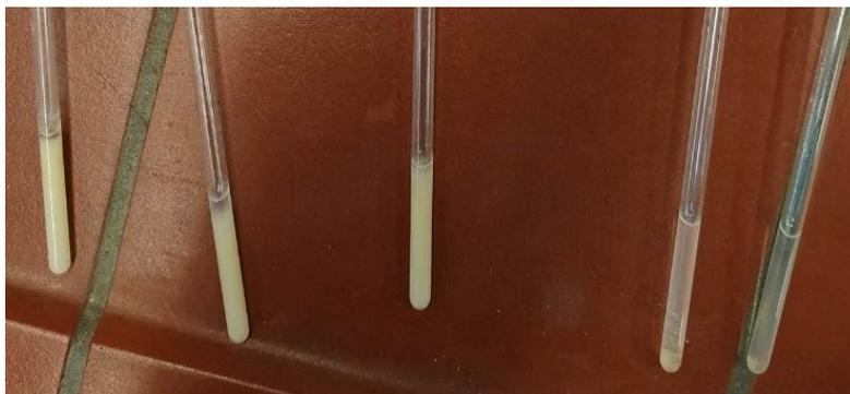
**Figure 4.10.:** Samples taken from reaction carried out in the flask after time steps 1h to 7h (left to right).
