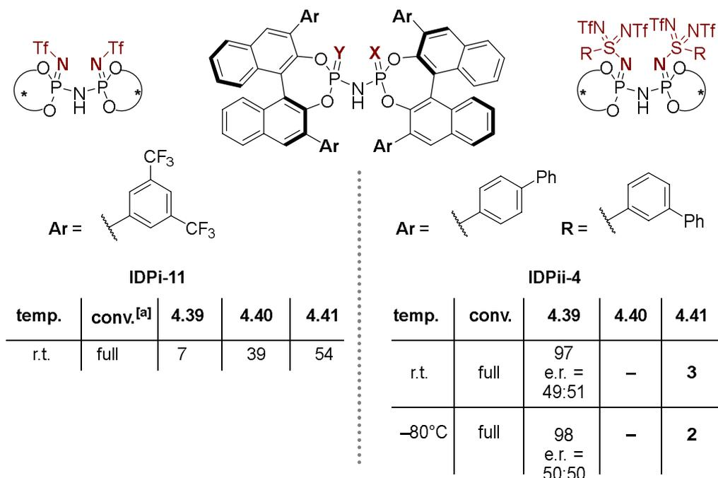
Scheme 53: The hydridodehydroxylation in the presence of **IDPi-11** and **IDPii-4** catalysts.
