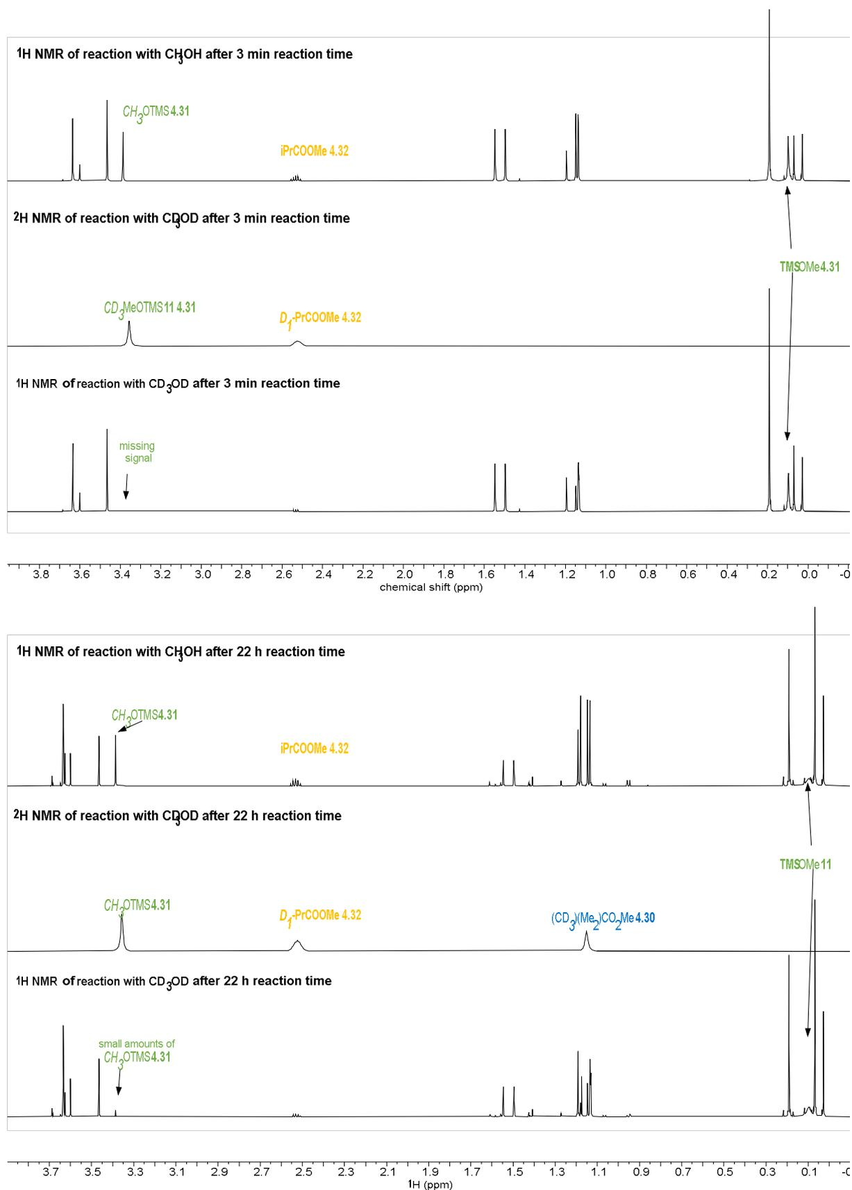
Figure 11: <sup>1</sup>H and <sup>2</sup>H-NMR-spectra after 3 min and 22 h reaction with MeOH and MeOH-d<sub>4</sub>.
