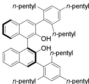
The BINOL has been synthesized based on example **4.1**. FCC-conditions: (gradient: hexanes / CH<sub>2</sub>Cl<sub>2</sub> 95:5 to 80:20); 71% yield (yellowish oil).
