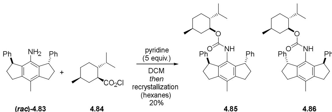
Scheme 63: Resolution of aniline **4.83** via derivatization with menthylchloroformate **4.84**.
