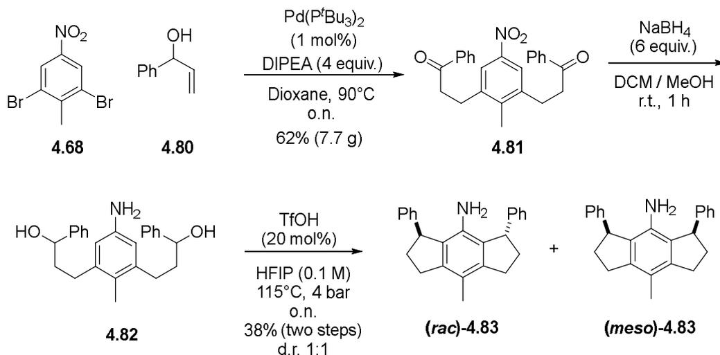
Scheme 62: Synthesis of tetrahydroindacene-derived aniline **4.83**.
