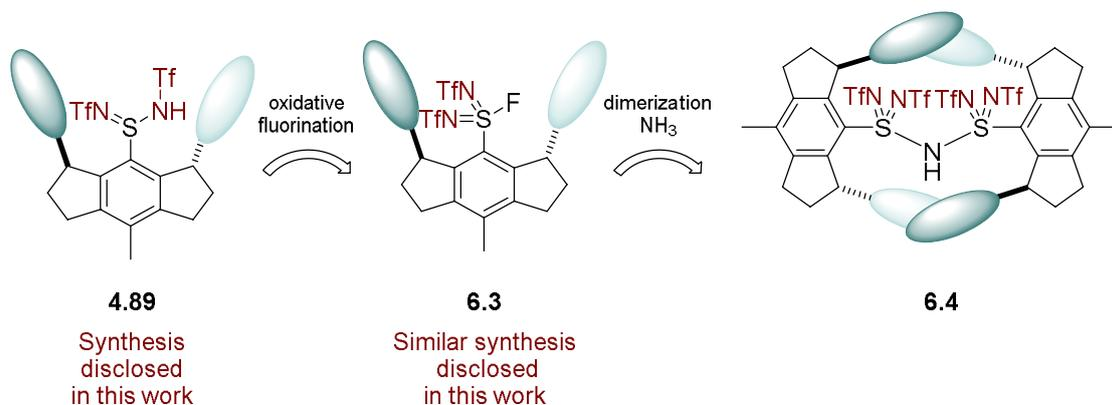
Figure 17: Dimerization of tetrahydroindacene-derived bis(iminosulfonyl)sulfonyl fluoride **6.3** to access a new class of dimeric catalyst motifs based on the disulfonimide core (**6.4**).
