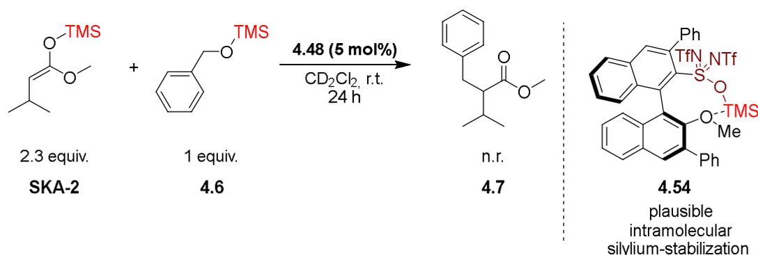
Scheme 57: Selected example for the  $\alpha$ -alkylation of silyl ketene acetal **SKA-2**. Proposed reactivity decrease due to intramolecular silylium ion stabilization with the adjacent methoxy moiety (right).
