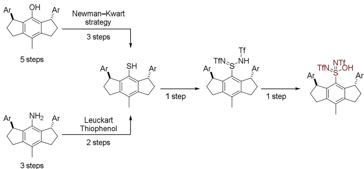
*Scheme 69: Synthesis toward tetrahydroindacene-derived bis(trifluoromethylsulfonylimino)sulfonic acid.*
