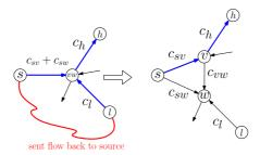
Fig. 5. Rerouting flow in the directed case.
