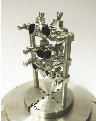
**Figure 2.17: Coaligned multi-crystal assembly for neutron scattering experiments.** The single crystals of nearly cylindrical shape with a diameter of around 4 mm and a length of up to 1.5 cm are individually fixed in aluminium clamps which are attached to two aluminium rods. This setup enables each crystal to be rotated individually around two axis for easy coalignment.
