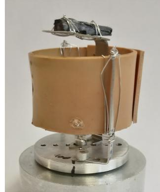
**Figure 5.5: Mounted crystal of  $\text{Sr}_2\text{Ru}_{0.95}\text{Co}_{0.05}\text{O}_4$ .** A big single crystal of the 5% Co doped compound is mounted on an aluminium sample holder for neutron scattering experiments. A LiF shield is used to decrease background by avoiding scattering stemming from aluminium.
