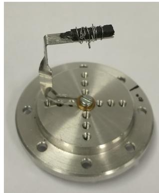
**Figure 3.4:** Mounted  $\text{Ca}_2\text{Ru}_{1-y}\text{Ti}_y\text{O}_4$  ( $y = 0.01$ ) crystal. The big 1% Ti doped  $\text{Ca}_2\text{RuO}_4$  and essentially untwinned crystal ( $V \approx 150 \text{ mm}^2$ ) is mounted and oriented for the neutron scattering experiment.
