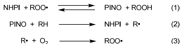
Scheme 2-27: General mechanism for the NHPI catalyzed autoxidation reaction.
