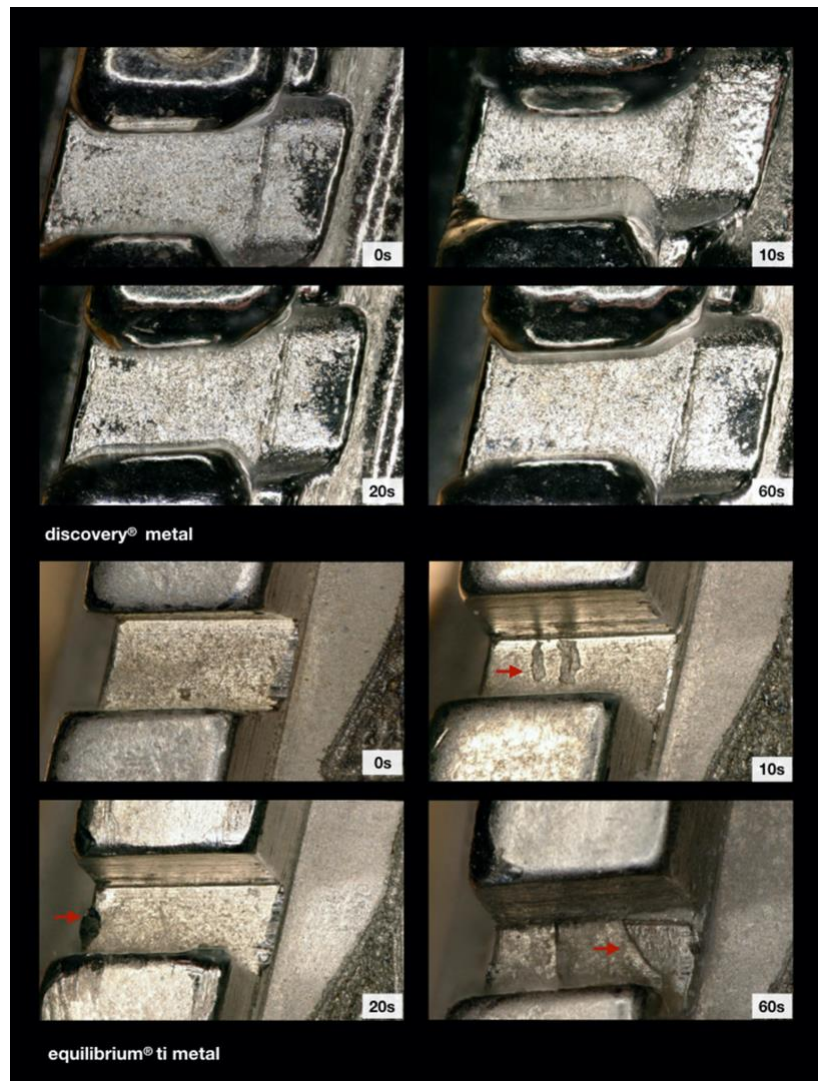
Fig. 8 Illustration of the mesial slot properties of both metal brackets with respect to exposure time. Chipping effects ( arrows ) were mainly observed for the titanium bracket. Light microscope images, 200× magnification
