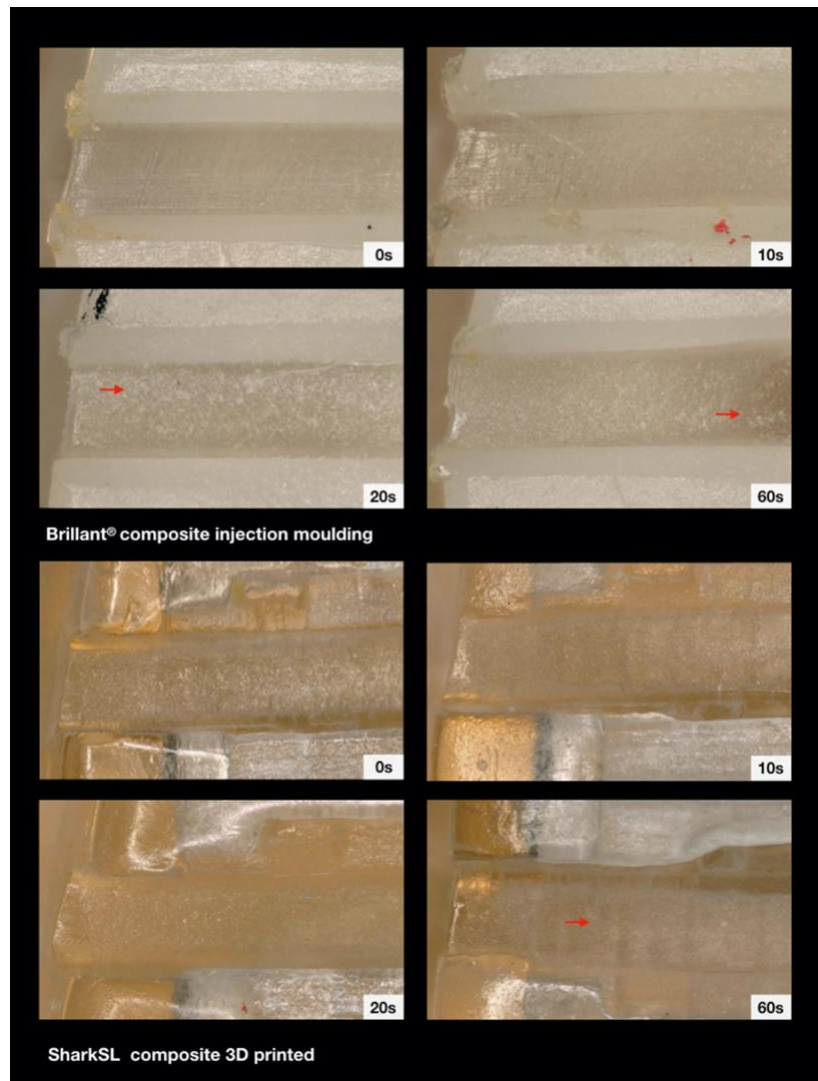
Fig. 6 Illustration of the mesial slot properties of both polymer brackets with respect to exposure time. Increasing exposure time resulted in slight abrasion ( arrows ) which was mainly observed in the Brillant® brackets. Light microscope images 200x magnification
