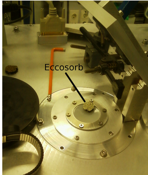
Figure 4.21: The eccosorb marks the position where the center beam comes out of the cryostat in both cases, CR and CT. The diameter of the entrance window is 35 mm.
