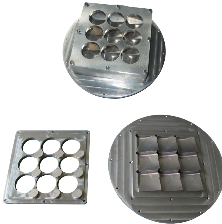
Figure 4.12: Pictures of the 1.1 THz Array Receiver FPU optics built in aluminum and based on the CHARM concept [Lüthi et al., 2006]. Top: The FPU optics ensemble. Bottom: The two plates with all the illumination (left) and collimation (right) mirrors, each is built out of one aluminum block in a machining cycle. The spacer frame that keeps both plates at a distance of 40 mm is not presented separately. The diameter of the circular plate is 175 mm.
