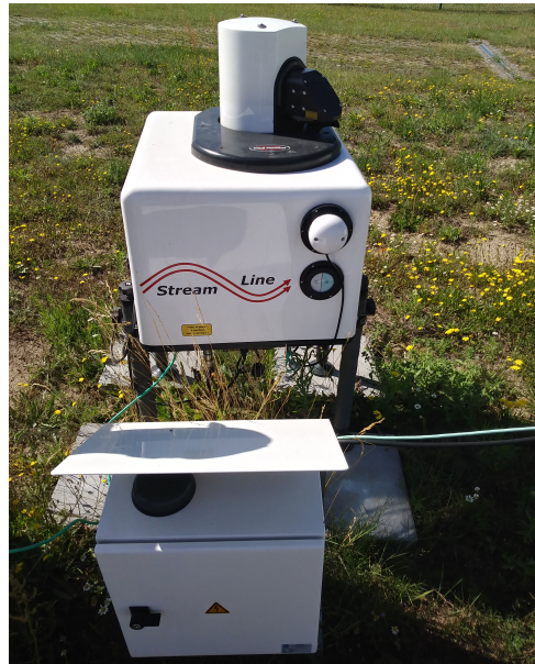
Figure 3.2: A StreamLine DWL, manufactured by Halo Photonics, that was used in this study and within the FESSTVaL campaign. The author made the photo on July 22, 2020 at the Boundary Layer Field site in Falkenberg, Germany.
